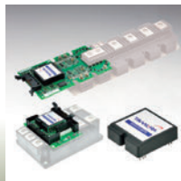
Power modules, current sensors, and gate drivers
